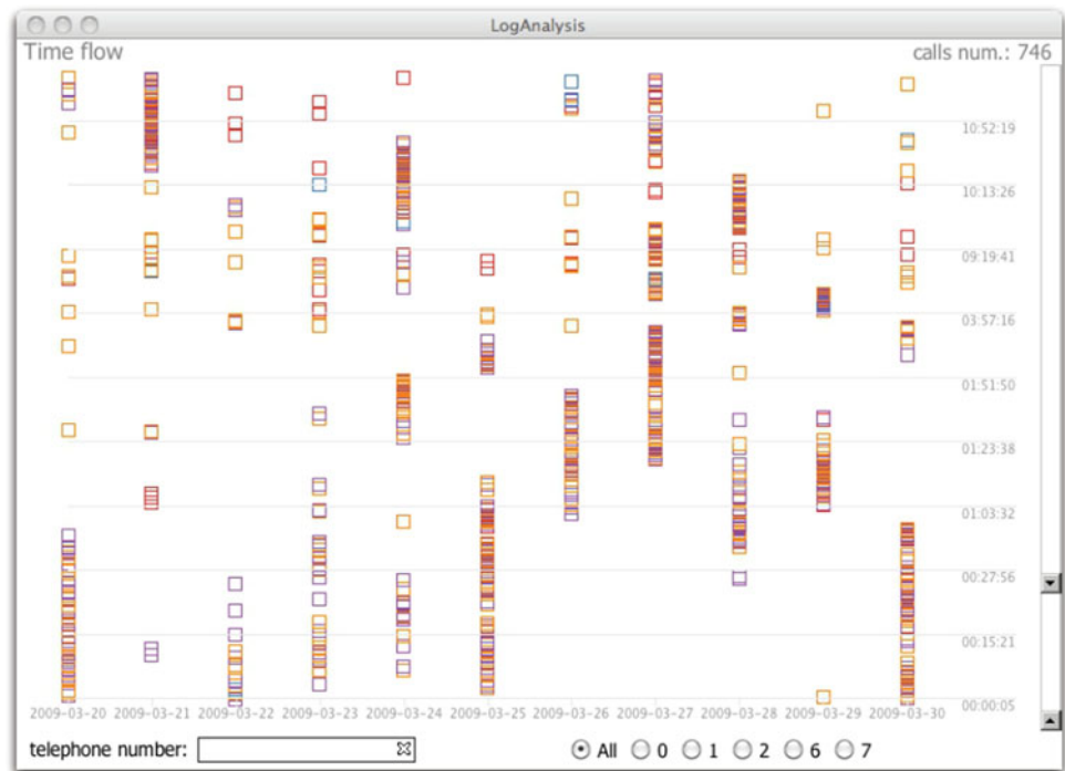
Fig. 9 The time flow analyzer tool. This tool is helpful to consider the time-dependence of events (i.e., phone calls) in a specific time window and it is crucial in order to highlight phone call cascades during criminal events
